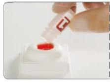
Pour the entire contents to the center of the mebran unit well. The sample should be absorbed through the membrane in less than 30 seconds.
