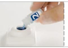
inverting to mix the solution thoroughly. Open the vial and add the entire contents to Membrane Unit well. the center of the membrane Unit well. Wait for absorption.
